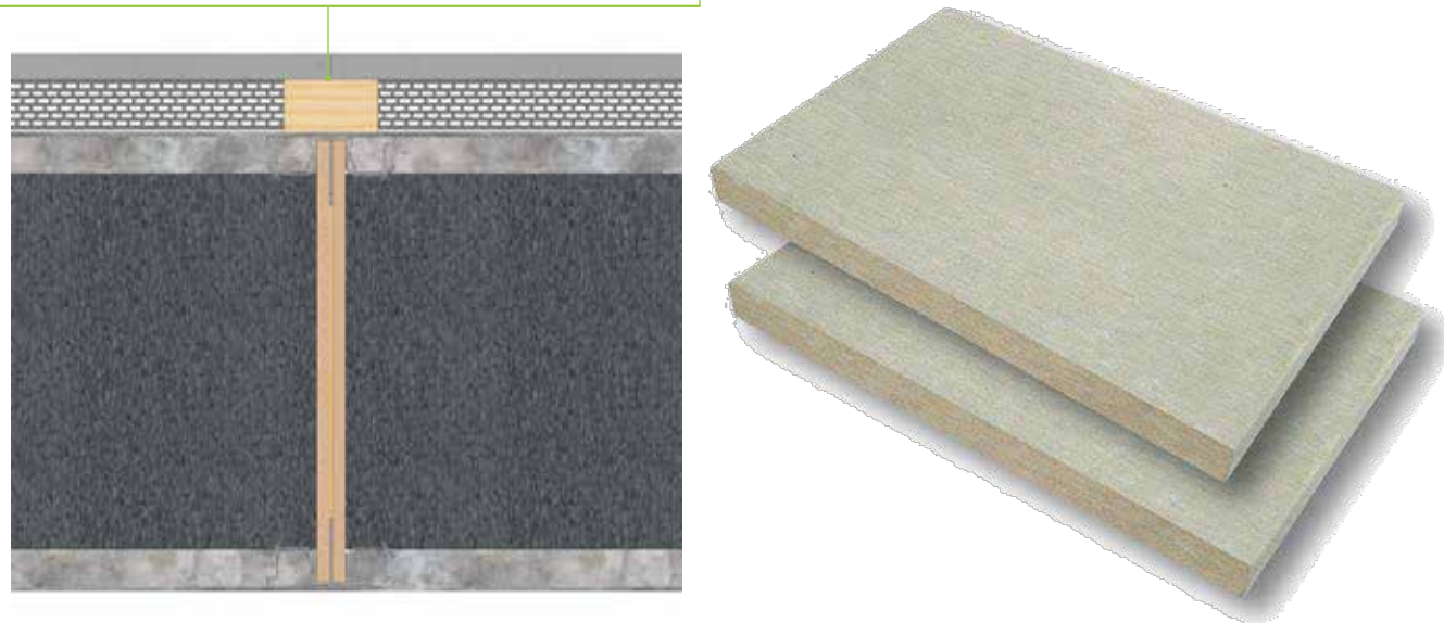
Calcium silicate board fixed to timber batten
